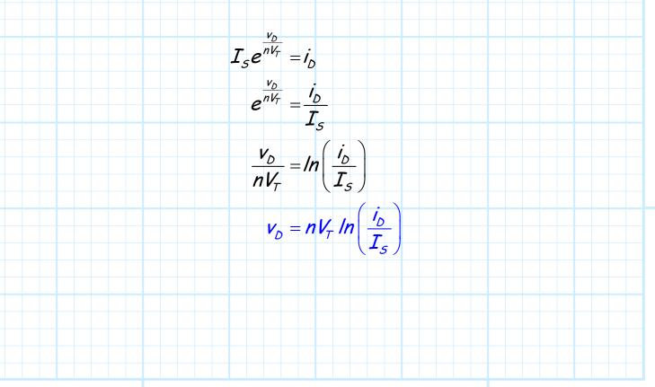
Now, say a voltage  $v_1$  across some junction diode results in a current  $i_1$ . Likewise, **different** voltage  $v_2$  across this same diode a diode of course results in a **different** current  $i_2$ . We can define the difference between these two voltages as  $\Delta v = v_2 - v_1$ , and then using the above equation can express this voltage difference as:
