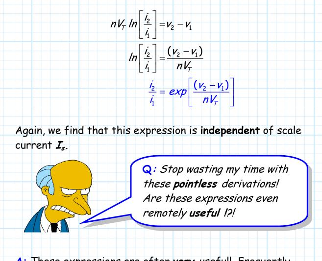
A: These expressions are often very useful! Frequently, instead of explicitly providing device parameters n and  $I_s$ , a junction diode is specified by stating n, and then a statement of the specific diode current resulting from a specific diode voltage.
